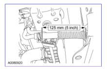
NOTICE: The filter has a bypass valve in it. The red arrow on the filter indicates the direction of the fluid flow through the filter. The filter must be installed in the fluid cooler return line with the red arrow pointing away from the transmission fluid cooler and toward the transmission (the return line has fluid coming out of the cooler going to the transmission). If the fluid filter is not installed correctly, it will cause internal transmission damage.
