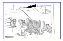
6. Clean a visible section of the transmission fluid pan and install the sticker.
